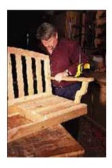
The back of the arm is simply screwed in place through the back stile, while the support is attached to the arm and seat with dowels and polyurethane glue. Notice the foamy squeeze-out of the glue at the joints.
