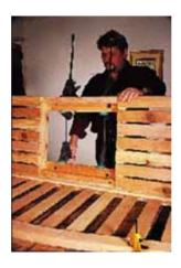
With the notches cut in the support cleats, the two pieces can be glued in place in the seat frame
